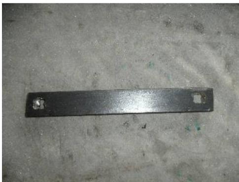
Two 1/4 Whitworth open-enders got from local hardware shop were cut in half & welded together to give me a deeper grip. Next a piece of bar 1" x 3/8" about 9" long, drilled to make the spanner a snug fit square at one end & angled at the other end - I can now get on all the bolts in situ & have double the purchase on the nuts.
