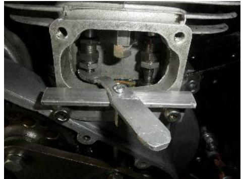
Next I got a cheap set of feeler gauges, cut the two ones I needed shorter & cut a square hole in the sides of them & after cleaning off the burs with a file they fit into their respective places with no hands!. So that leaves two hands to do the adjustment & locknuts, a pleasure doing that job now.
