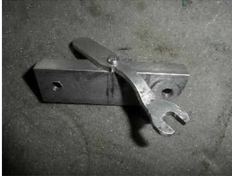
A small length of aluminium angle with a crude spanner fashioned out of the same ali to stop the cam followers turning that was screwed to the angle & fixed in the middle so it swings over to grab the other one.
